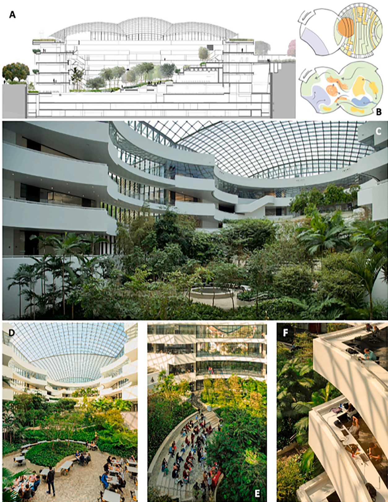
Fig. 1. (A) Longitudinal section of the building (West-East); (B) Atrium garden - schematic plans: above: initial design from the architecture team; below: redesign proposal by the landscape team, with planting areas in green, living areas in yellow, restaurant area in light blue, amphitheater in orange and with arrows indicating the expansion of the garden towards the restaurant area; (C) Atrium garden seen from an upper level. Photo: Manoel D. Leão Neto; (D) General view of the atrium garden, with the restaurant in the foreground. Photo: Fernando Guerra; (E) Atrium garden - amphitheater. Photo: Fernando Guerra; and (F) Studying areas surrounding the atrium garden. Photo: Fernando Guerra.
